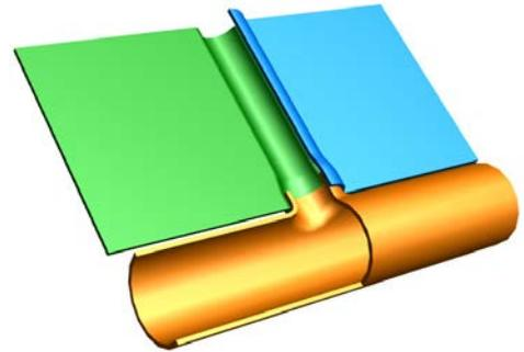
**Figure 2: Header tube with collar produced by hydroforming (left) and basic connection concept with roll-bond absorber (right); source: Fraunhofer IWU**
