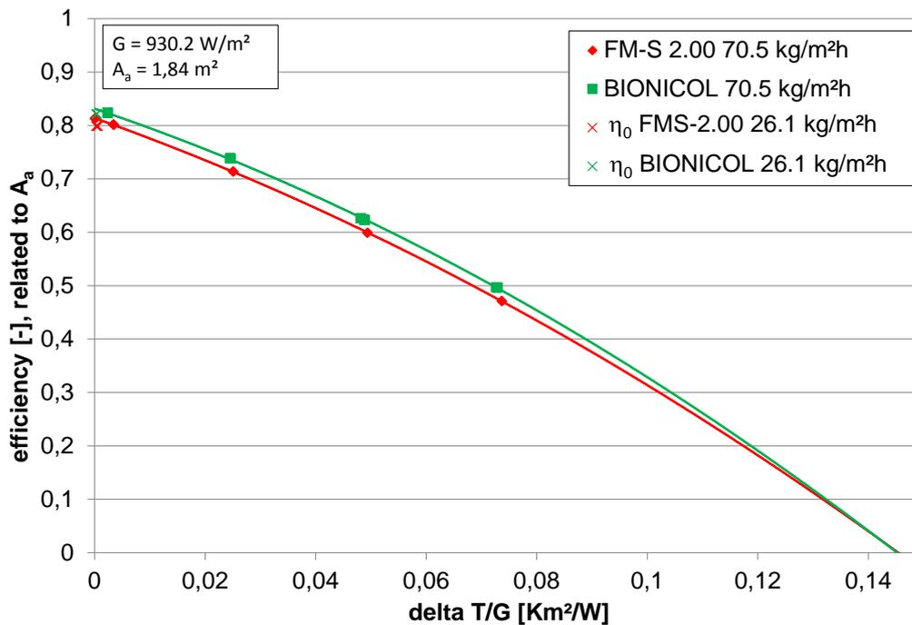
Figure 5: Efficiency curves of FM-S 2.00 and BIONICOL collector at standard flow rate as well as  $\eta_0$  at low flow rate of 26.1 kg/m<sup>2</sup>h (with reference to the aperture area of the collector)
