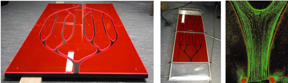
**Figure 1: Specimen (“Small absorber”) built as layer system from black PP, fluorescent PMMA and transparent PMMA cover (left), specimen inserted in custom-built sump attached to the hydraulic system (middle) and streamlines made visible by hydrogen bubbles (right)**
