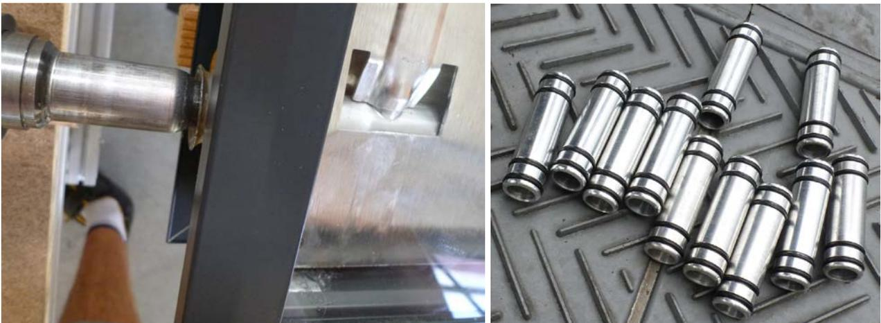
**Figure 3: BIONICOL header tube end-forming for the connector part (left) and aluminium connectors used in the field test systems (right)**
