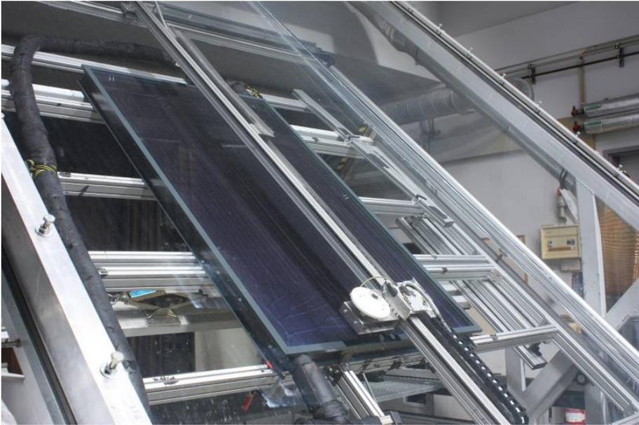
Figure 7: BIONICOL collector installed on test rack of solar simulator at FRAUNHOFER ISE
