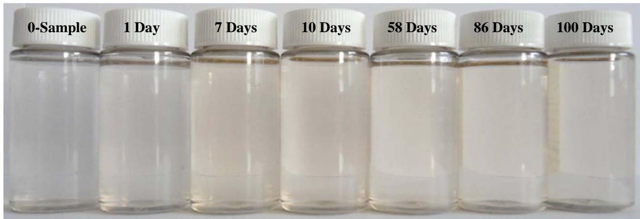
**Figure 5: Appearance of selected fluid samples taken during corrosion test under stagnation conditions**
