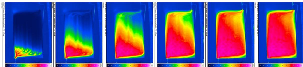
**Figure 4: Thermography sequence of absorber with FracTherm® channel design**
