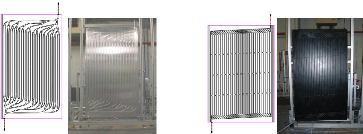
Figure 1: Roll-bond panels with FracTherm<sup>®</sup> (left) and CGA design (right)
