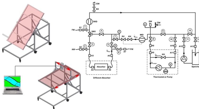
**Figure 5: Draft and hydraulic scheme of the fluid dynamics test facility**
