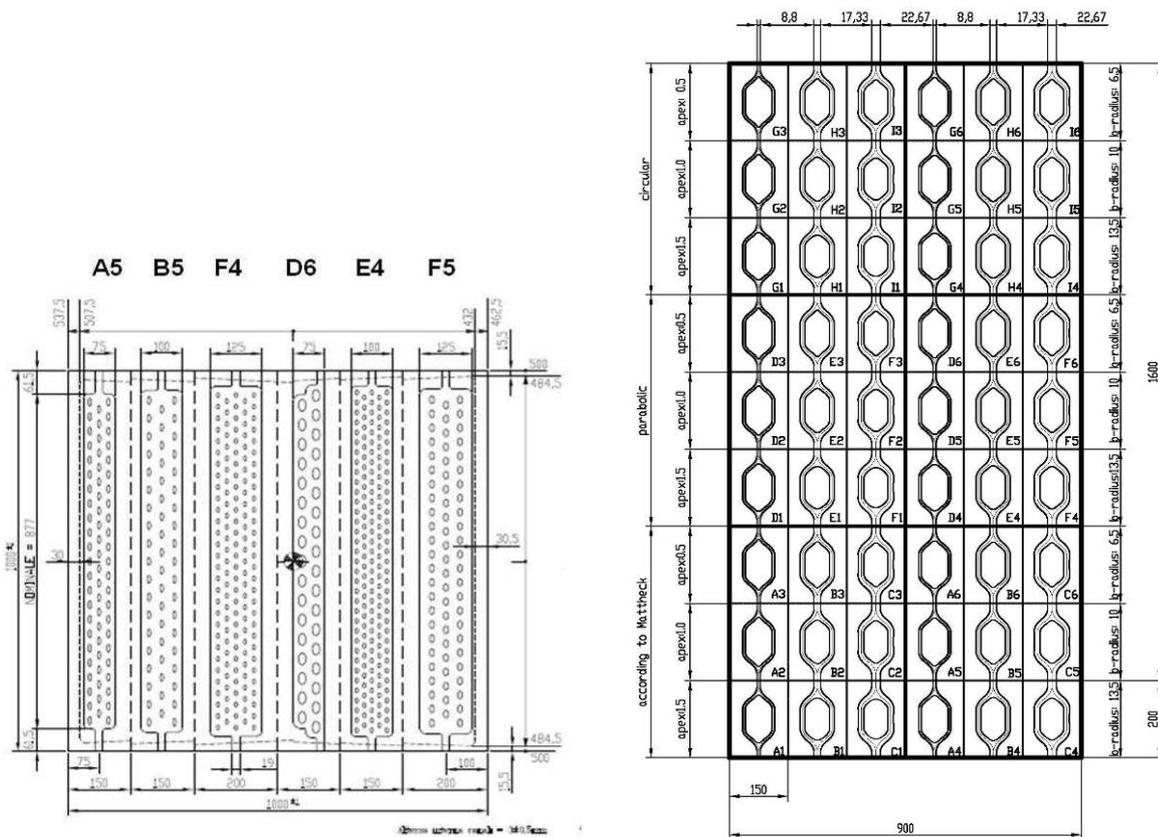
Figure 1: Roll-bond samples with different header (left) and bifurcation (right) geometries
