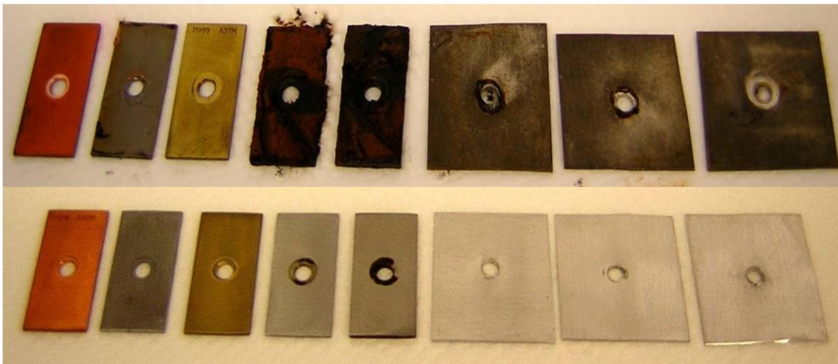
**Figure 6: Appearance of metal specimens after ASTM D1384 before cleaning / weighing (top: fluid without corrosion inhibitors, bottom: fluid with corrosion inhibitors)**
