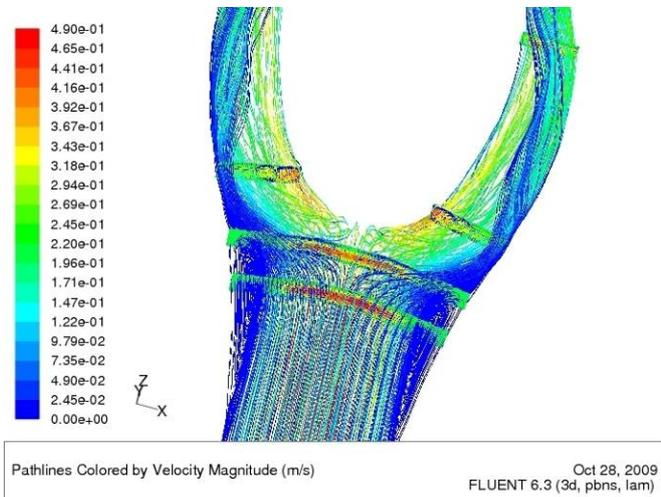
Figure 4: Streamlines of fluid flowing around a FracTherm<sup>®</sup> bifurcation (3D CFD simulation)
