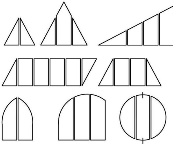
**Figure 7: Possible non-rectangular collector shapes**
