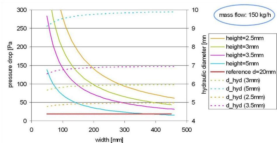
Figure 3: Pressure drop of rectangular headers in comparison with 20 mm tube
