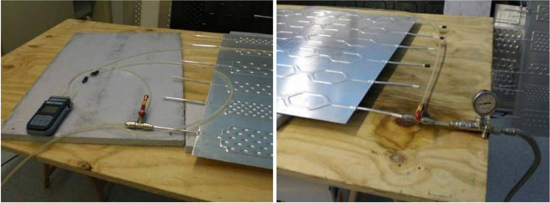
Figure 2: Pressure drop test of roll-bond samples
